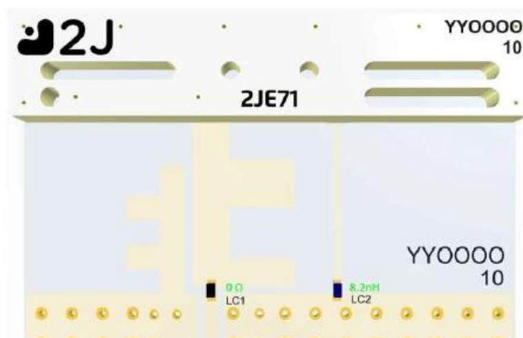
3D View of matching components and recommended values (LC1=0 Ohm, LC2=8.2 nH)
